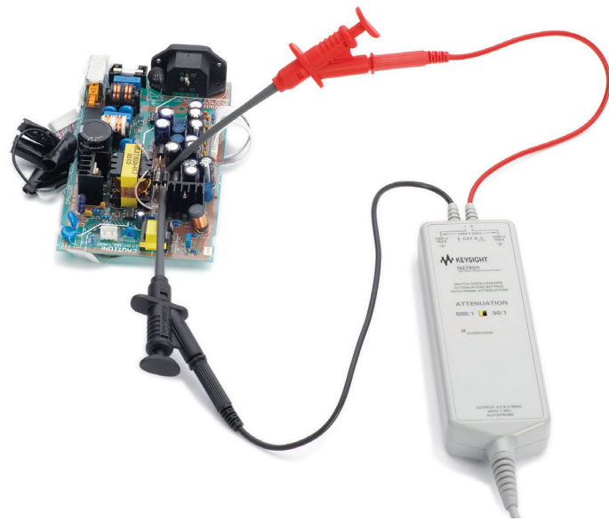
Figure 15. Versatile probe tip accessories allow you to access small or large components in tight places.
